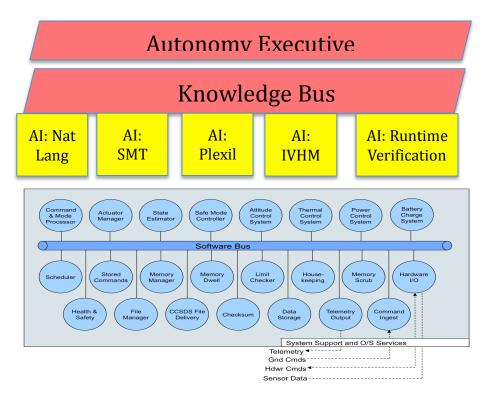
Figure 1: Block Diagram of AOS Architecture
